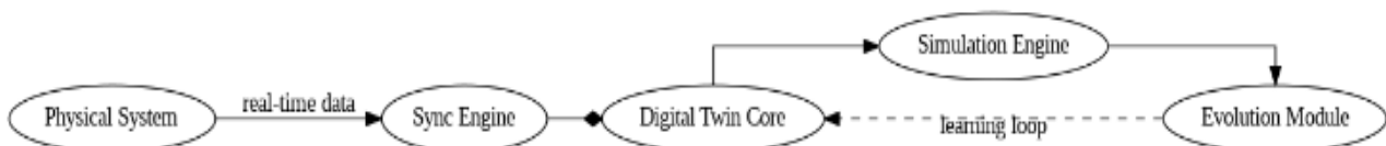
FIGURE 3. BIDIRECTIONAL EVOLUTIONARY DIGITAL TWIN SYSTEM.
