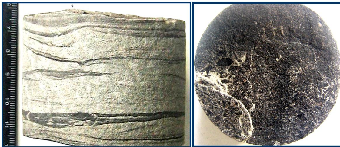
Figure 1. Gray, light grey sandstone with numerous inclusions of plant detritus, North Berdakh deposit, borehole no. 10, int. 2340-2346 m.
