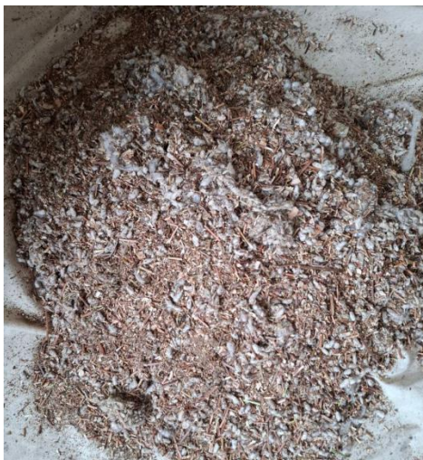
Fig. 2. Appearance of waste from the waste bunker of the sections of the UHK cotton cleaning unit
