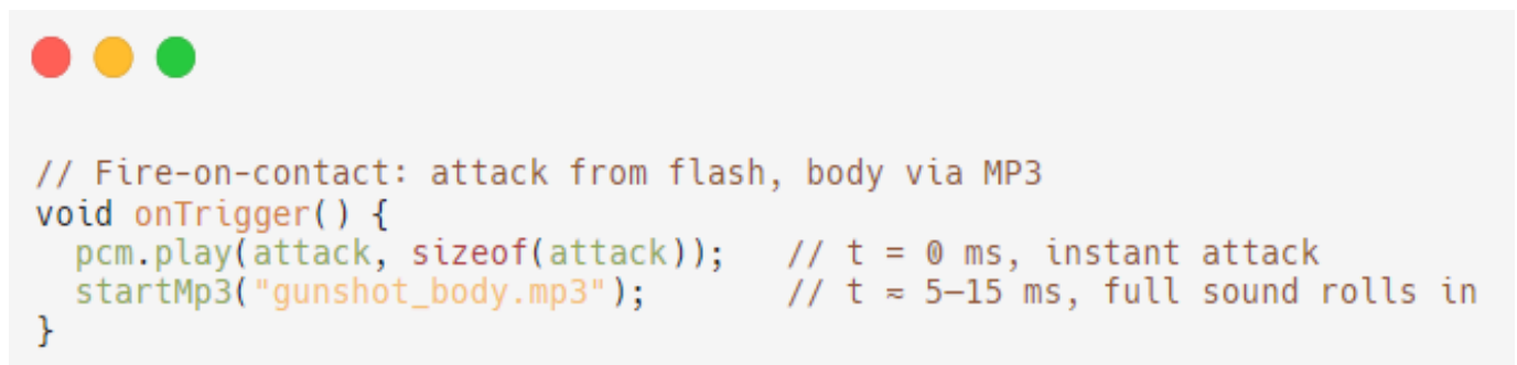
Fig. 2. Algorithm for reducing auditory delay using a hybrid PCM/MP3 method
