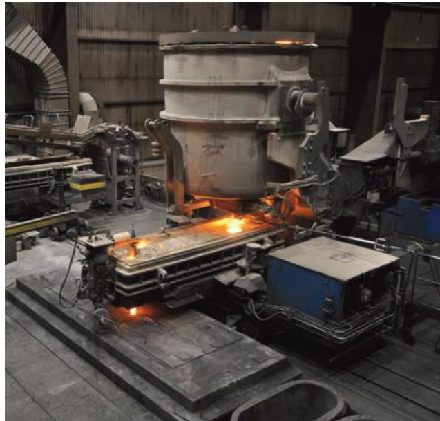
Figure 4. Continuous casting. Turred with ladle and tundish, from which the molten steel is led down into the mould by the submerged entry nozzle (SEN).
