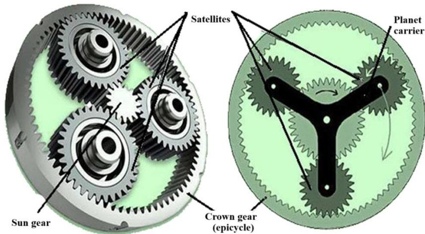
Fig. 1. Planetary gear diagram
