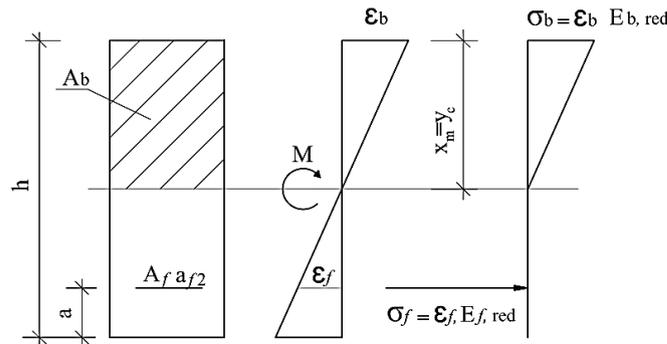
**Figure 1. A scheme for calculating the deformations of an element with the given cross-section and cracks under the action of a bending moment in the stressed-strained state.**
