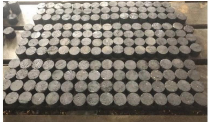
(b) Partial coal samples prepared by processing
