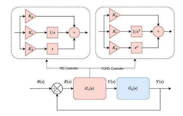
Three different tuning methods are used to tune the PID controller: Ziegler-Nichols (ZN) method, Cohen-Coon (CC) method, and Internal Model Control (IMC) method. The ZN method involves step testing the process and determining the ultimate gain and ultimate period to calculate the proportional, integral, and derivative gains. The CC
