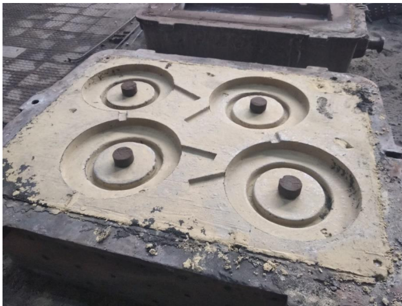
Figure 2. Sand-clay mold to get the disk cast
