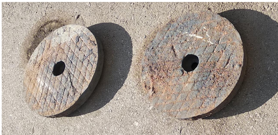
Figure 4. Appearance of disk cast cast in sand-clay mold
