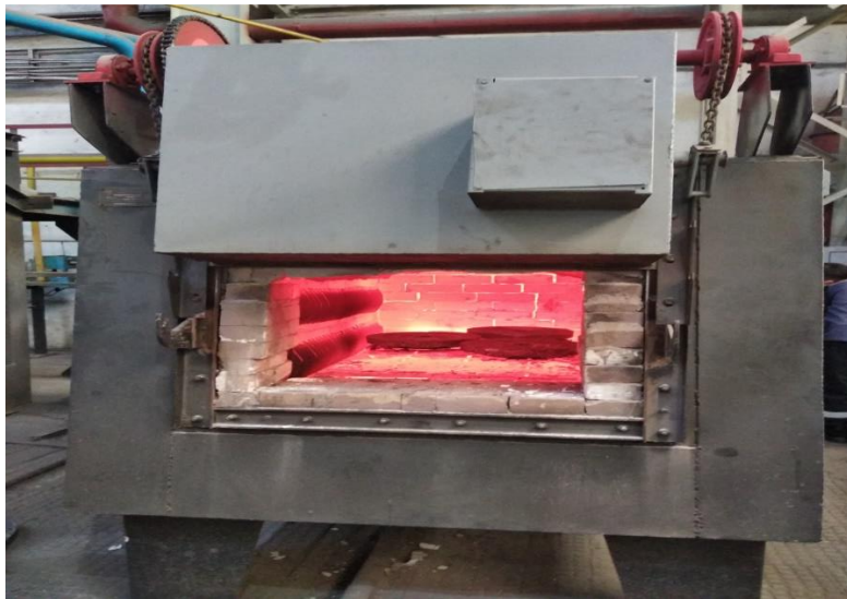
Figure 3. SNOL - 7.2 / 1100 muffle furnace for heat treatment of samples
