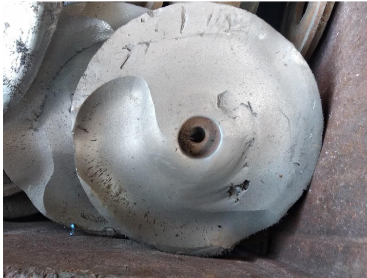
Figure 1. Appearance of a disk cast that has become unusable
