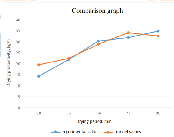
Figure 4. Comparison graph of drying productivity values found by the model and experimentally determined.
