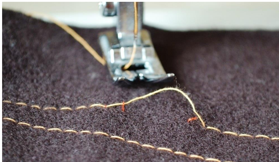
Picture 1. Seam defect
