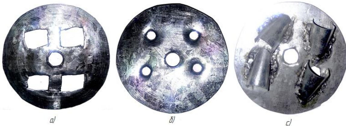
Figure 5. Constructions of plates selected for the experiment A rectangular hole is drilled. b) - a round hole is drilled. c) - an oval hole is drilled and a guide device is installed
