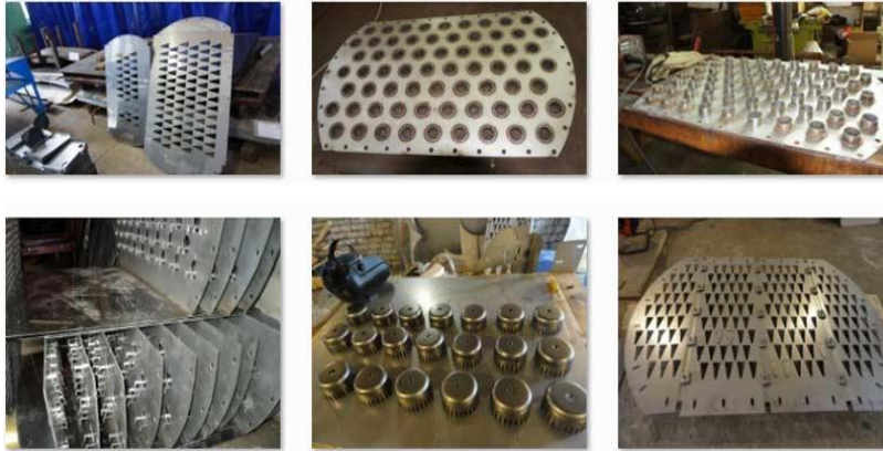
Figure 1. Structures of rectification columns used in the production of acetic acid.
