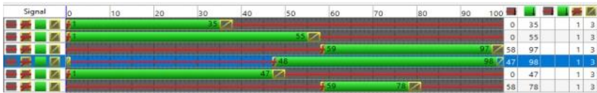
Figure 8. Duration of the green light for the current state
