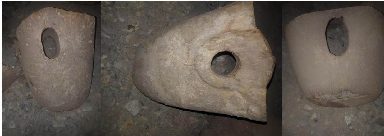
Figure 2. Perforation of HITACHI EX-1200 excavator bucket teeth due to erosion
