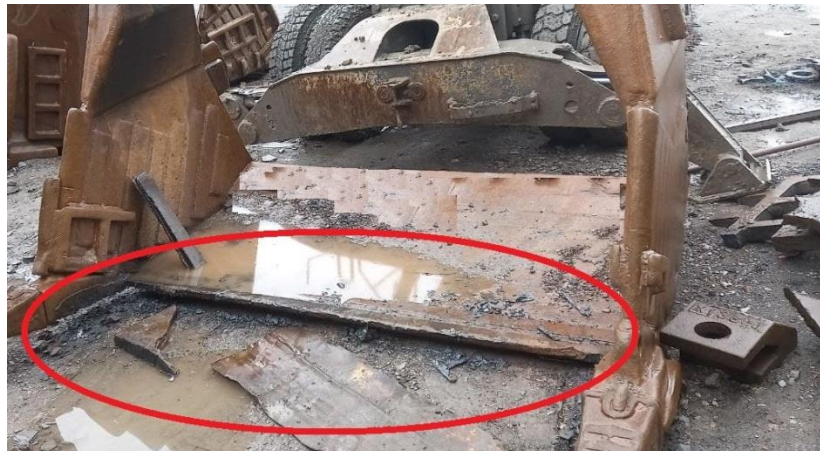
Figure 3. The fracture state of the cutting edge of the jaw
