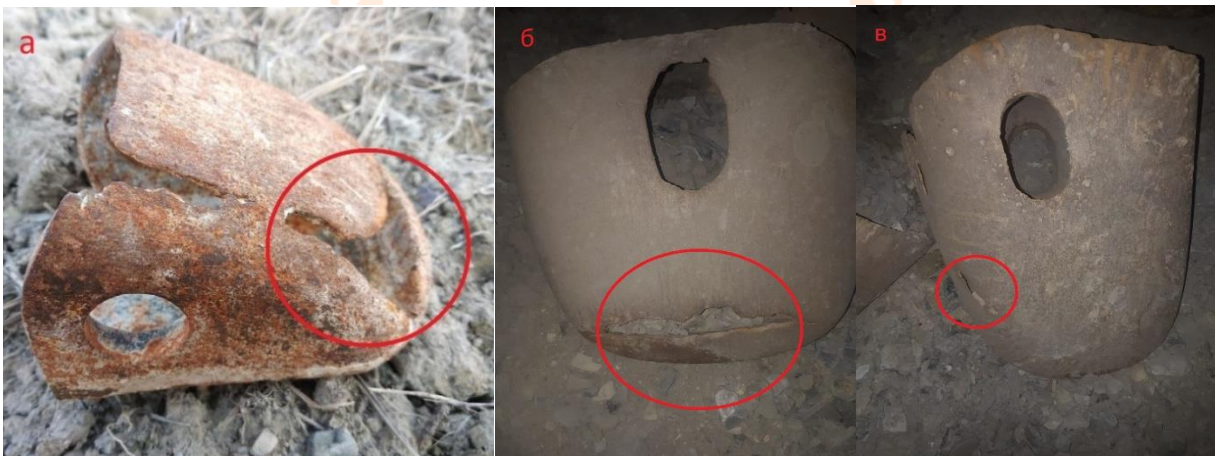
Figure 2: Perforations in the bucket teeth of the HITACHI EX-1200 excavator as a result of erosion: a - front and side perforation; б - front perforation; в - side perforation
