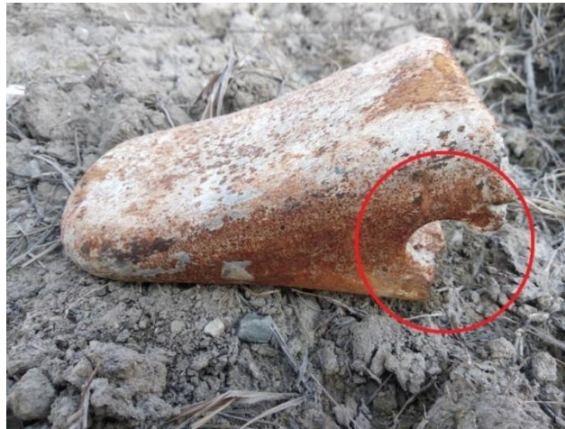
Figure 3: Fracture of the teeth of the backhoe bucket
