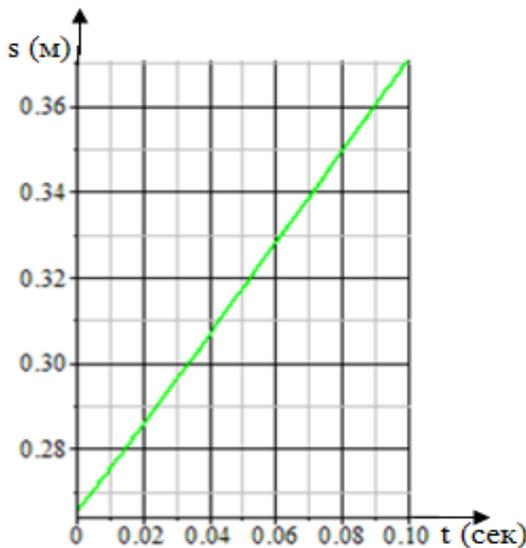
Fig. 5. The law of movement of seeds along the section of the DE grate in the course of time.
