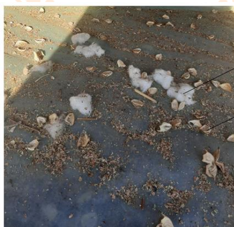
Fig. 5. Weed impurities and volatiles of raw cotton, fallen out under the roller table rollers 1 - cotton wedges, 2 - weeds.
