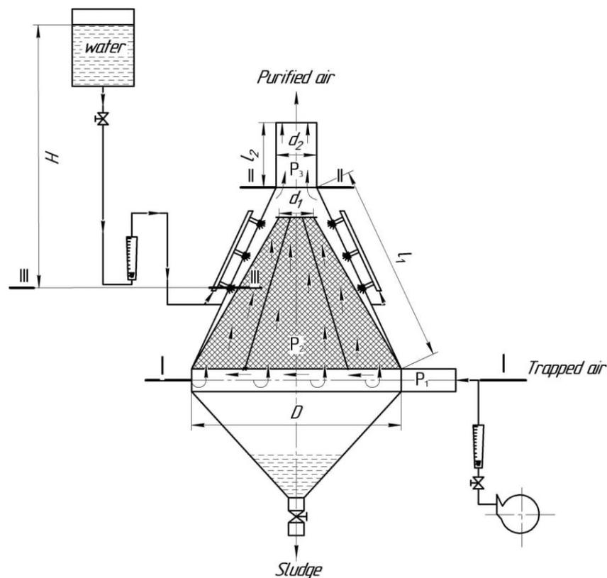
Figure 2. The calculation scheme of the device
