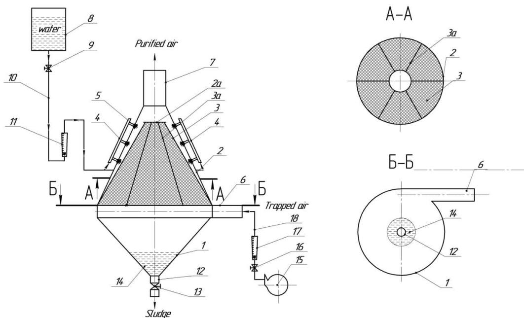
1 – bottom conical sludge bath, 2 – upper conical cleaning chamber, 3 – conical grid, 3a – grid support, 4 – sprinkler nozzle, 5 – water distribution pipe, 6 – dust gas inlet pipe, 7 – purified gas outlet pipe, 8 – water tank, 9 – water jet, 10 – water pipe, 11 – water rotameter, 12 – sludge drain pipe, 13 – sludge jug, 14 – sludge, 15 – dust fan, 16 – dust air jet, 17 – dust Rotameter, 18 – dust gas transmission pipe.
