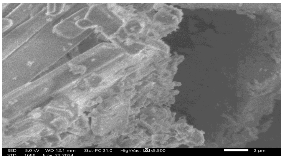
Fig. 3 SEM image of non-heat-treated phosphogypsum.
