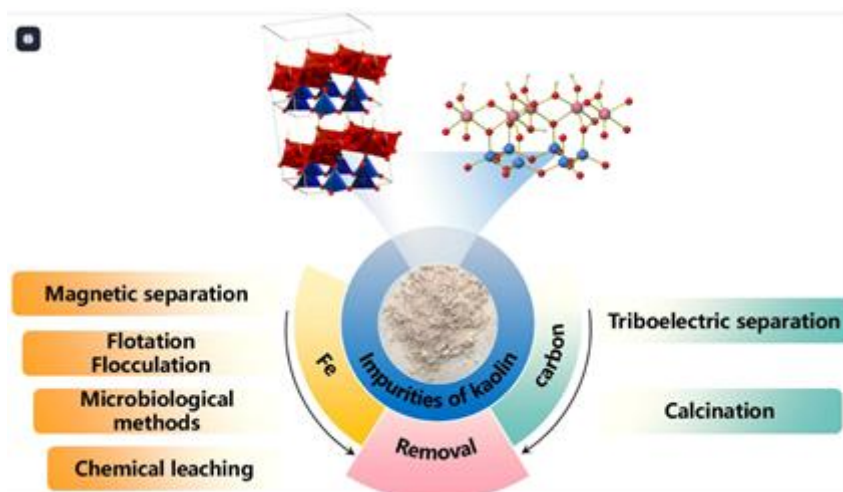
Figure 2. Methods of Kaolin Purification
