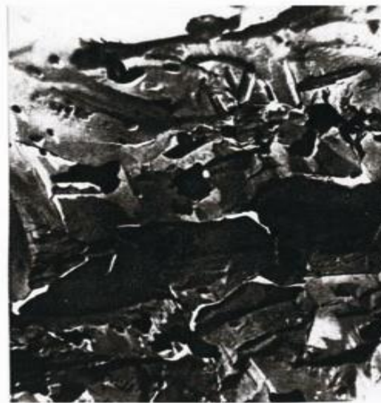
Rice. 3. Micrographs of replicas from the surface of the SIC clinkers with KH = 0.667 and nS = 1.5 (b) and 2.0 (c), synthesized at 1200°C. x 5300
