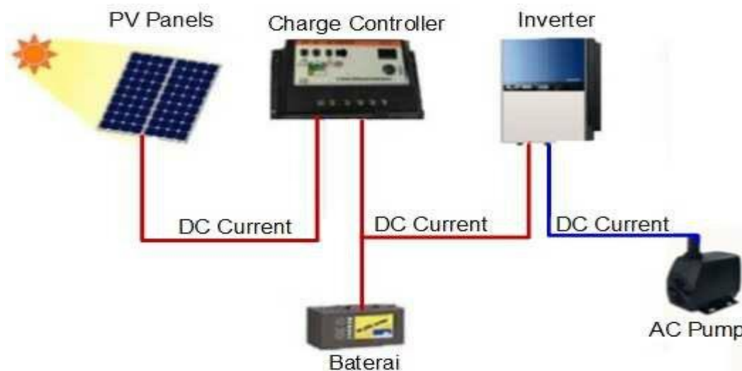
Figure 3 - Schematic diagram of a solar-powered hydroponic pump [3]
